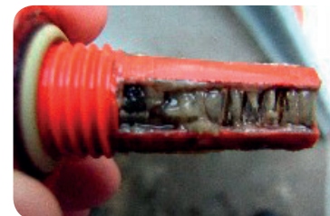
Nipple clogged with biofilm
